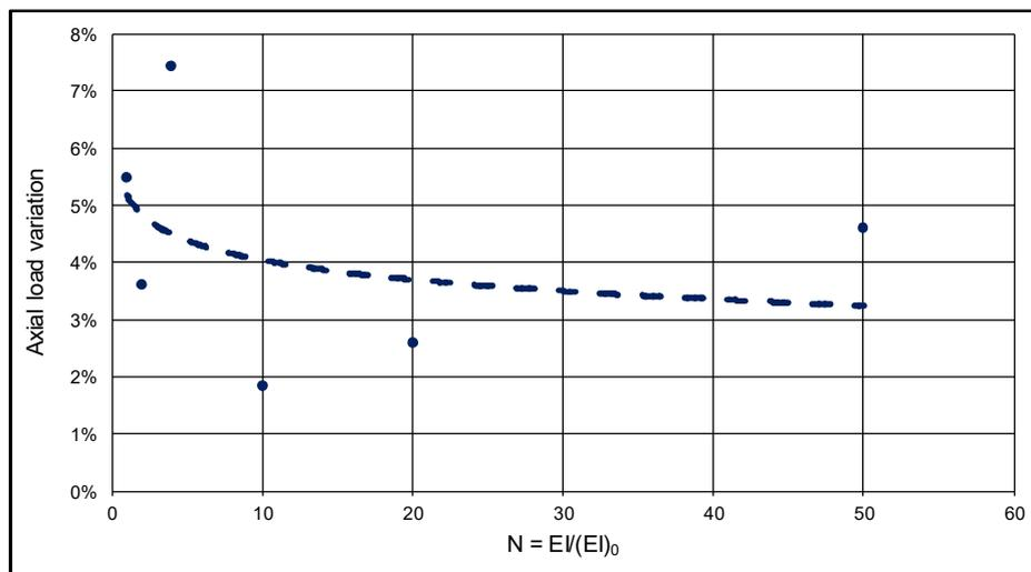
Figure 9: Correlation between flexural stiffness and axial load change
