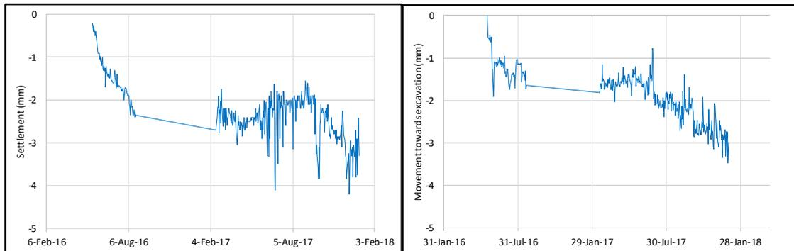
Figure 6: Monitoring results (prism mounted about top of l-shaped wall)
