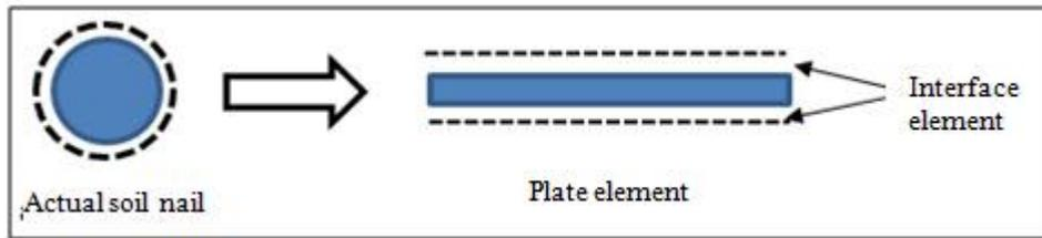
Figure 4: Circular shaped soil nail modelled with rectangular plate element
