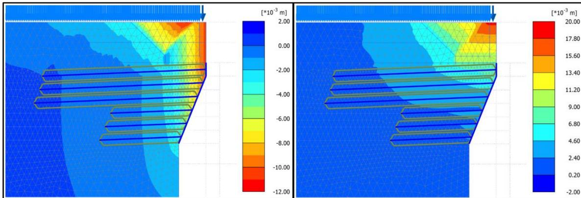
Figure 5: Contours of settlement (maximum 12 mm) and movement towards the excavation (maximum 18mm)
