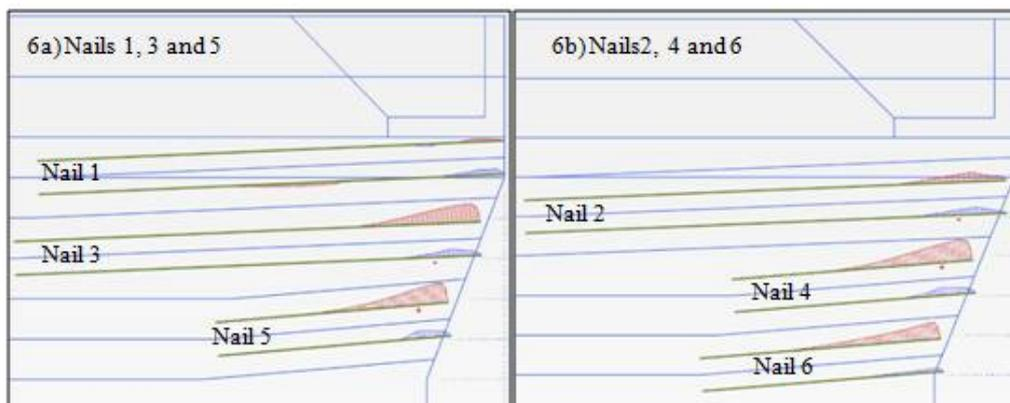
Figure 7: Relative movement on interface elements between nails and surrounding rock (maximum 2.5 mm)
