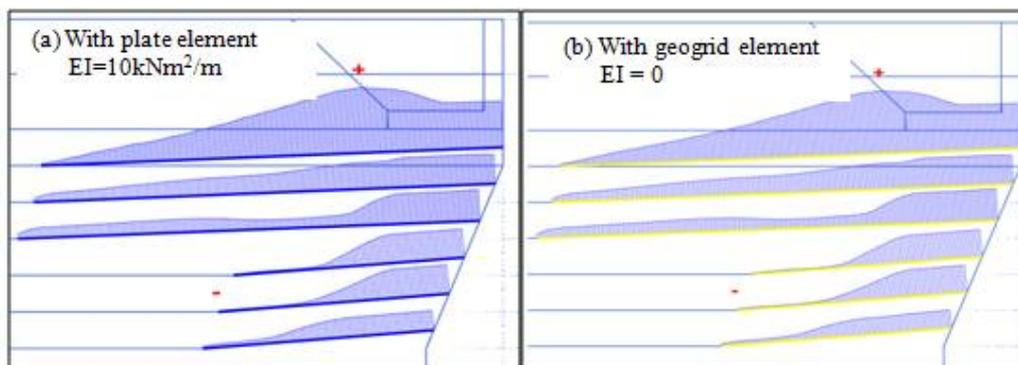
Figure 8: Soil nail axial load with “plate element” and with “geogrid element”
