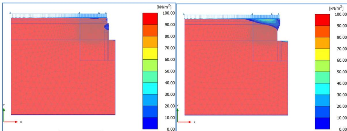
Figure 2: Zone of minor principle stress in tension – vertical excavation and excavation with undercut
